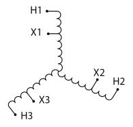
Three Phase Autotransformer with a capacity of 112.5kVA, transforming 416Y Volts to 347Y Volts
