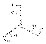
Three Phase Autotransformer with a capacity of 15kVA, transforming 600Y Volts to 277Y Volts
