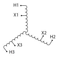
Three Phase Autotransformer with a capacity of 600kVA, transforming 277Y Volts to 110Y Volts
