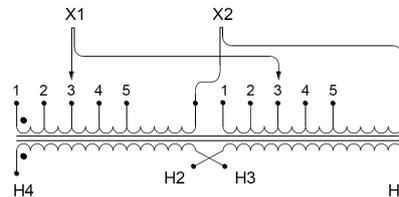
Single Phase Isolation Transformer with a capacity of 15kVA, transforming 120 Volts to 220/440 Volts
