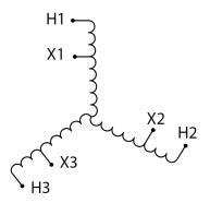
Three Phase Autotransformer with a capacity of 500kVA, transforming 240Y Volts to 575Y Volts
