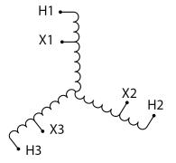
Three Phase Autotransformer with a capacity of 225kVA, transforming 110Y Volts to 415Y Volts
