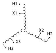
Three Phase Autotransformer with a capacity of 112.5kVA, transforming 550Y Volts to 110Y Volts
