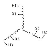
Three Phase Autotransformer with a capacity of 75kVA, transforming 415Y Volts to 600Y Volts
