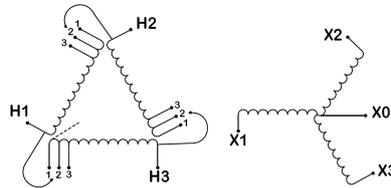
Three Phase Encapsulated Isolation Transformer with a capacity of 9kVA, transforming 480 Volts to 380Y/220 Volts
