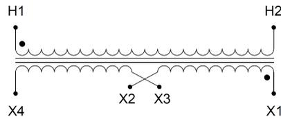
Single Phase Control Transformer with a capacity of 100VA, transforming 480 Volts to 240/480 Volts
