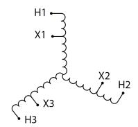
Three Phase Autotransformer with a capacity of 3kVA, transforming 240Y Volts to 440Y Volts
