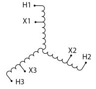
Three Phase Autotransformer with a capacity of 3kVA, transforming 277Y Volts to 460Y Volts
