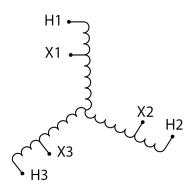
Three Phase Autotransformer with a capacity of 9kVA, transforming 115Y Volts to 400Y Volts
