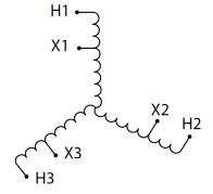
Three Phase Autotransformer with a capacity of 15kVA, transforming 200Y Volts to 220Y Volts
