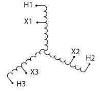
Three Phase Autotransformer with a capacity of 15kVA, transforming 200Y Volts to 550Y Volts
