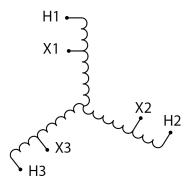
Three Phase Autotransformer with a capacity of 75kVA, transforming 208Y Volts to 347Y Volts
