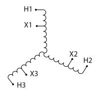
Three Phase Autotransformer with a capacity of 45kVA, transforming 380Y Volts to 480Y Volts
