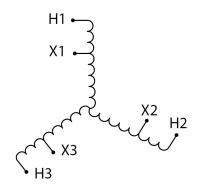
Three Phase Autotransformer with a capacity of 3kVA, transforming 115Y Volts to 277Y Volts
