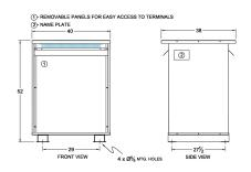
Three Phase Isolation Transformer with a capacity of 300kVA, transforming 347 Volts to 415Y/240 Volts
