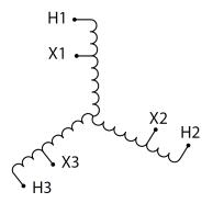
Three Phase Autotransformer with a capacity of 750kVA, transforming 208Y Volts to 277Y Volts
