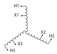
Three Phase Autotransformer with a capacity of 6kVA, transforming 115Y Volts to 220Y Volts
