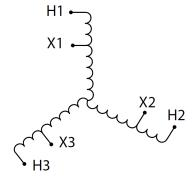
Three Phase Autotransformer with a capacity of 6kVA, transforming 347Y Volts to 240Y Volts
