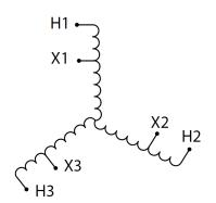
Three Phase Autotransformer with a capacity of 45kVA, transforming 110Y Volts to 440Y Volts
