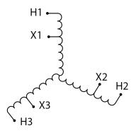
Three Phase Autotransformer with a capacity of 45kVA, transforming 115Y Volts to 277Y Volts
