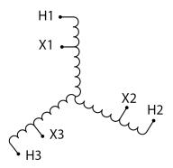
Three Phase Autotransformer with a capacity of 1500kVA, transforming 550Y Volts to 440Y Volts
