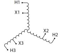
Three Phase Autotransformer with a capacity of 112.5kVA, transforming 120Y Volts to 110Y Volts
