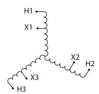
Three Phase Encapsulated Autotransformer with a capacity of 6kVA, transforming 600Y Volts to 208Y Volts
