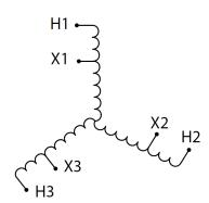
Three Phase Encapsulated Autotransformer with a capacity of 15kVA, transforming 480Y Volts to 240Y Volts
