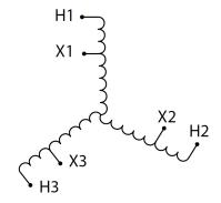
Three Phase Encapsulated Autotransformer with a capacity of 15kVA, transforming 480Y Volts to 240Y Volts
