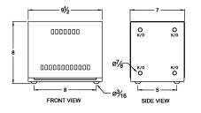
Single Phase Isolation Transformer with a capacity of 1kVA, transforming 208 Volts to 240/480 Volts
