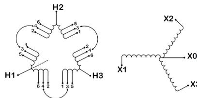
Three Phase Isolation Transformer with a capacity of 750kVA, transforming 550 Volts to 460Y/266 Volts
