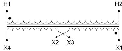
Single Phase Control Transformer with a capacity of 5000VA, transforming 208 Volts to 120/240 Volts
