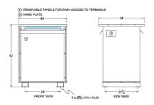
Three Phase Isolation Transformer with a capacity of 225kVA, transforming 416 Volts to 600Y/347 Volts
