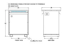
Three Phase Isolation Transformer with a capacity of 225kVA, transforming 600 Volts to 415Y/240 Volts
