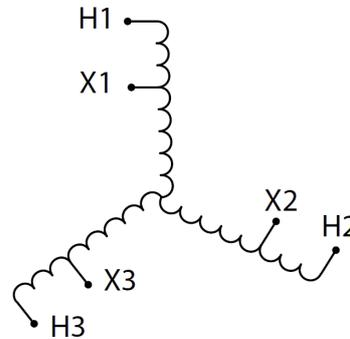
Three Phase Autotransformer with a capacity of 300kVA, transforming 110Y Volts to 460Y Volts
