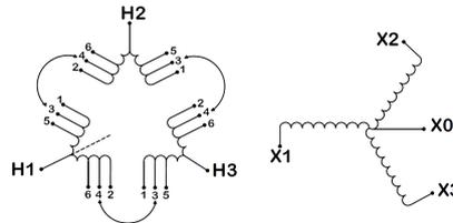
Three Phase Isolation Transformer with a capacity of 300kVA, transforming 600 Volts to 220Y/127 Volts
