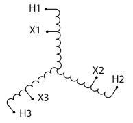
Three Phase Autotransformer with a capacity of 112.5kVA, transforming 110Y Volts to 600Y Volts
