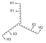
Three Phase Autotransformer with a capacity of 112.5kVA, transforming 416Y Volts to 115Y Volts
