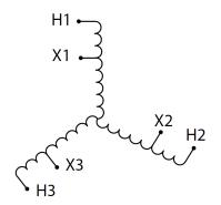
Three Phase Autotransformer with a capacity of 150kVA, transforming 115Y Volts to 400Y Volts
