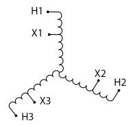
Three Phase Autotransformer with a capacity of 150kVA, transforming 347Y Volts to 115Y Volts
