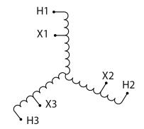
Three Phase Encapsulated Autotransformer with a capacity of 150kVA, transforming 600Y Volts to 208Y Volts
