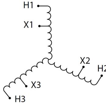
Three Phase Encapsulated Autotransformer with a capacity of 75kVA, transforming 480Y Volts to 208Y Volts
