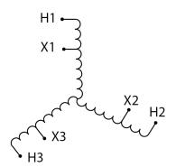
Three Phase Encapsulated Autotransformer with a capacity of 3kVA, transforming 480Y Volts to 208Y Volts
