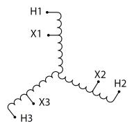
Three Phase Autotransformer with a capacity of 750kVA, transforming 600Y Volts to 110Y Volts
