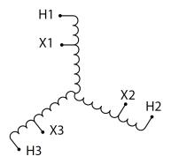
Three Phase Autotransformer with a capacity of 750kVA, transforming 110Y Volts to 575Y Volts
