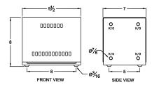
Single Phase Isolation Transformer with a capacity of 1kVA, transforming 220 Volts to 220/440 Volts
