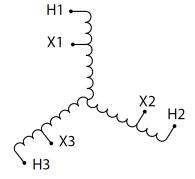
Three Phase Autotransformer with a capacity of 3kVA, transforming 400Y Volts to 600Y Volts
