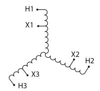
Three Phase Autotransformer with a capacity of 3kVA, transforming 347Y Volts to 400Y Volts
