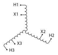
Three Phase Autotransformer with a capacity of 2500kVA, transforming 480Y Volts to 600Y Volts
