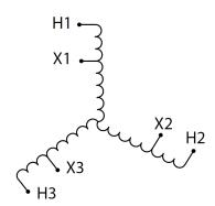
Three Phase Autotransformer with a capacity of 2500kVA, transforming 550Y Volts to 480Y Volts
